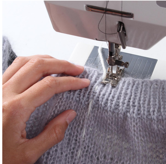
2. Sew 2 seams in zig-zag, one on each side of the marking thread.
